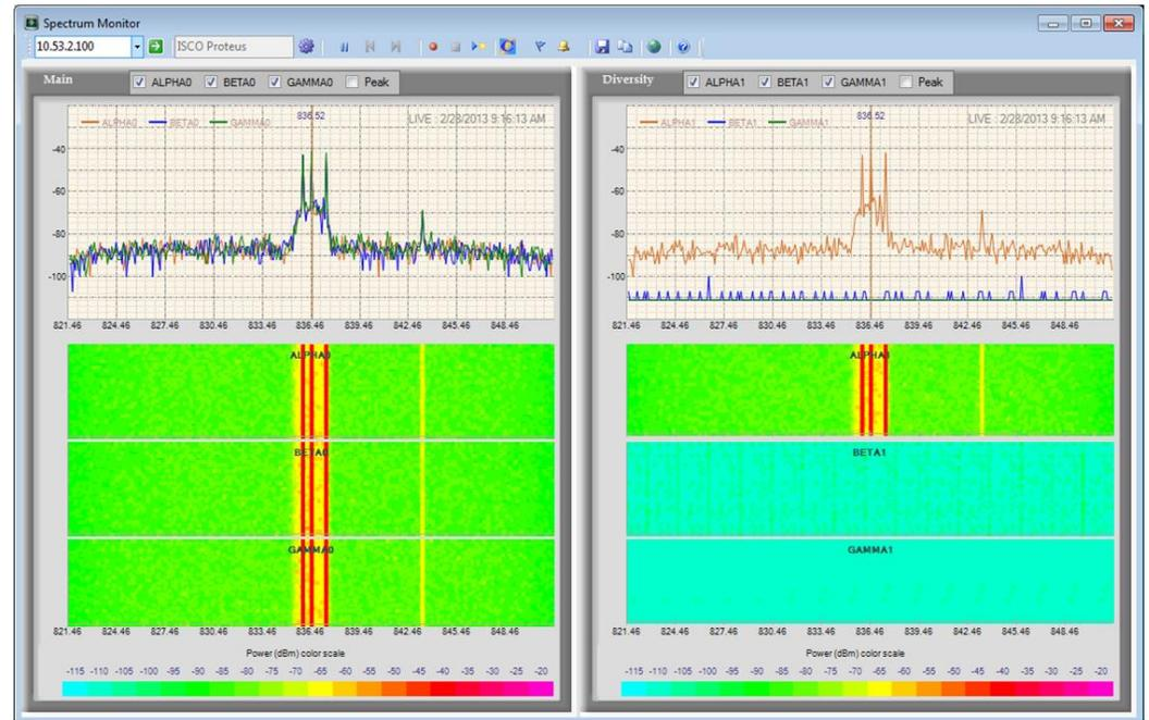
Three waterfall bands on the lower half of the screen correspond to each Alpha, Beta or Gamma face with the color indicating the magnitude of the power according to the scale at the bottom of the screen (red-pink indicates high power).
